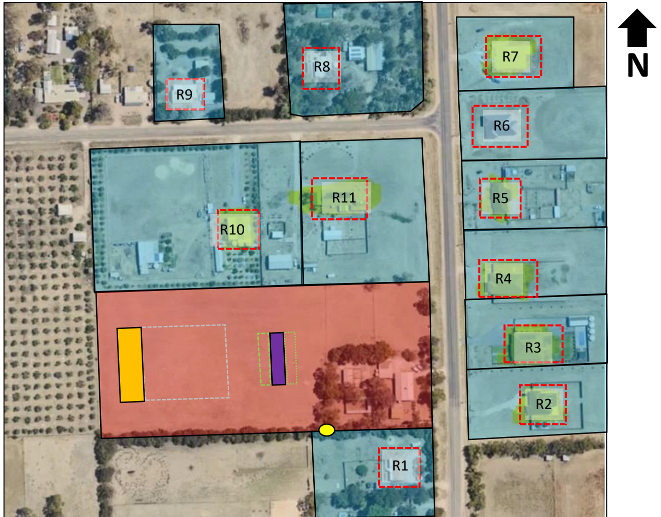
Figure 1 – Aerial Photo of the site, nearest noise sensitive receivers and noise monitoring location (Resourced from Google Maps)
