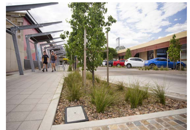
At Sixth Street, Murray Bridge, Jensen PLUS led a team to transform the streetscape into an attractive, green and functional street. Rain gardens pictured here catch stormwater and passively irrigate the new trees and plantings.
